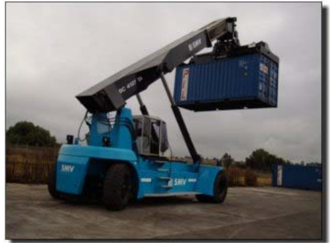
46 ton Stacker to move and stack containers
