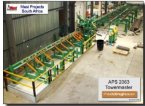
Angle Punch and cutting - CNC Machine
