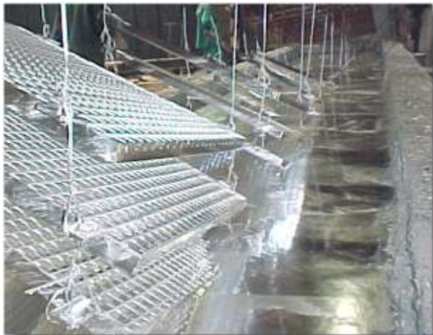
All parts are hot-dip galvanized
