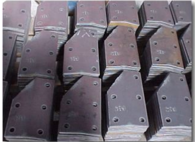
Gusset Plates ready for galvanizing
