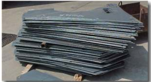
Profile cutting - platform sections
