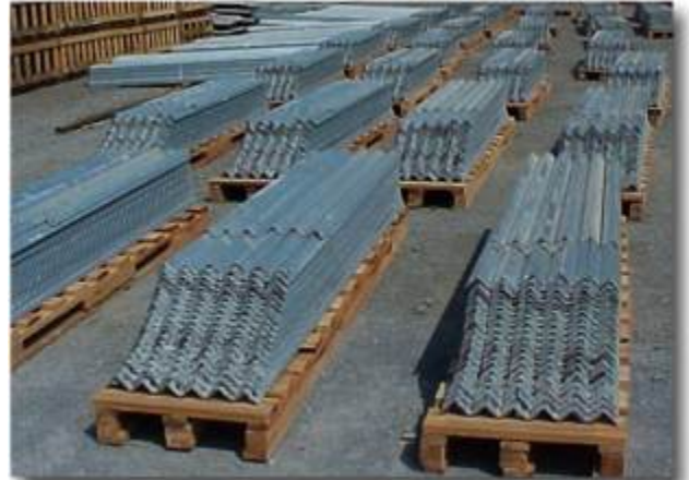
Horizontal and Diagonal tower members
