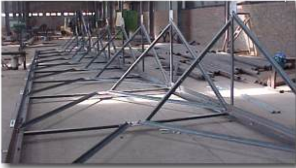
Proto-types are manufactured and approved - Angular Lattice BTS Rooftop Tower
