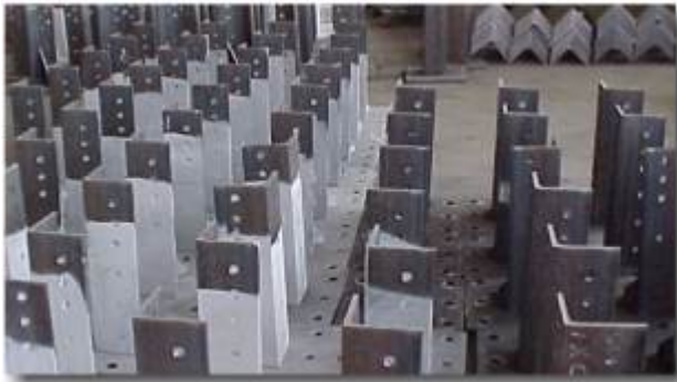
Welded Base Stubs ready for Galvanizing
