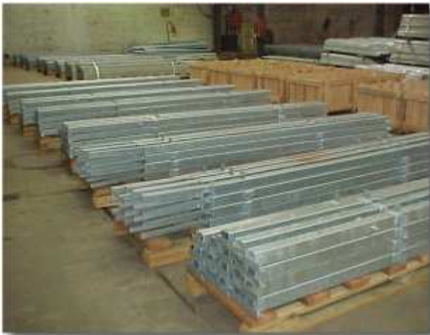
Palisade fencing posts packed
