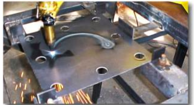
Manufacturing template plates
